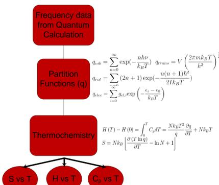
Figure 3: Thermochemistry calculation steps
