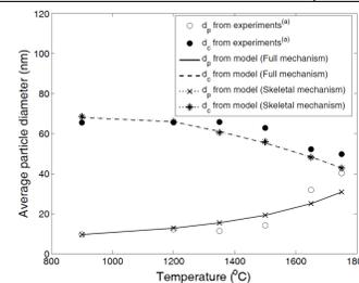
Figure 7: Change in average primary diameter ( $d_p$ ) and collision diameter ( $d_c$ ) with change in furnace temperature. Experimental values are from Seto et al [4].
