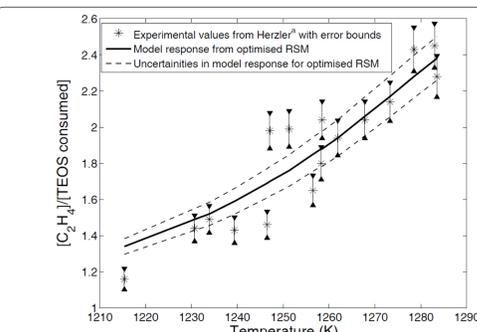
Figure 5: Optimised Model Response using Response surface methodology and associated uncertainties. Experimental values are provided by Herzler et al. [2]
