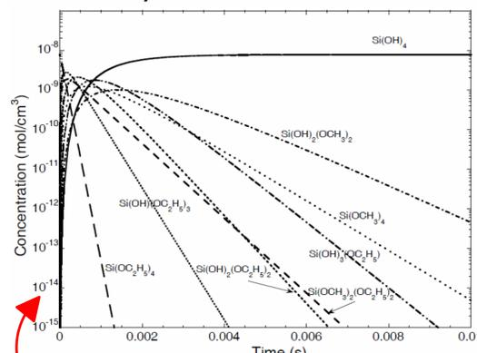
Figure 6: Reactor composition at  $T=1500$  K and  $P = 1$  atm.
